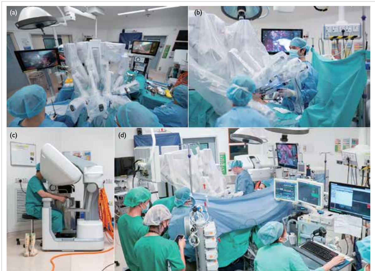
FIG 2. Intraoperative images of the Sentire Surgical System (CI000) during radical prostatectomy. (a) Robotic arms docked for the procedure. (b) Assistant surgeon position. (c) Surgeon Console. (d) Anaesthesiologist position
