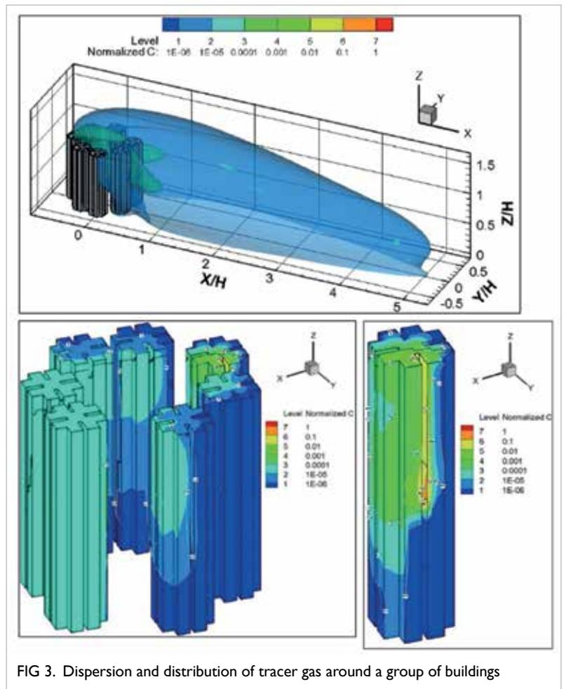
FIG 3. Dispersion and distribution of tracer gas around a group of buildings
