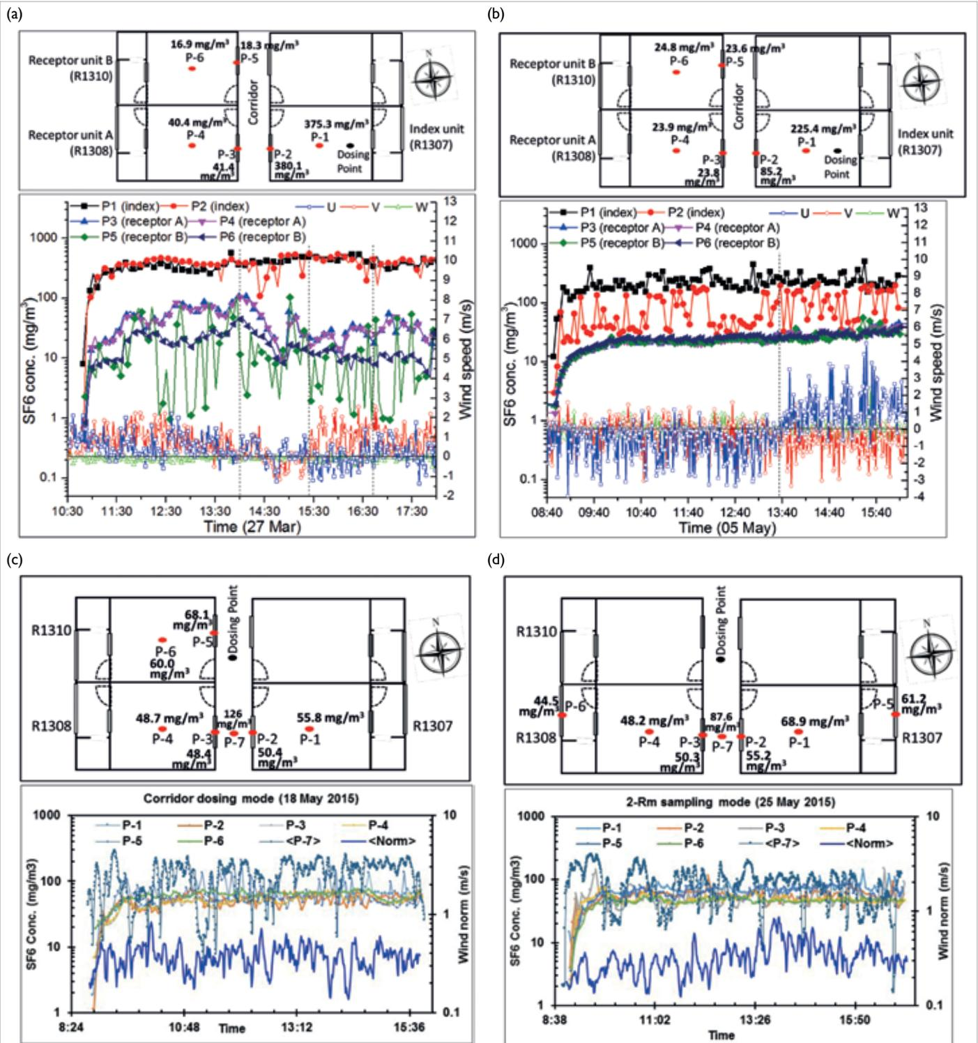
FIG 2. Mean SF<sub>6</sub> concentrations and concentration profiles: (a) closed window mode, (b) open window mode, (c) corridor dosing mode, and (d) 2-room mode
