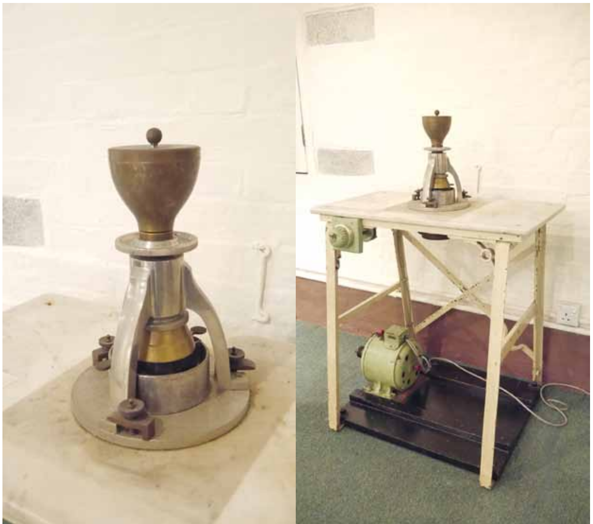
FIG. The triturator sits on a marble table. It is powered by a motor (green) connected to an electrical outlet (photos taken by Prof Harry Wu)
