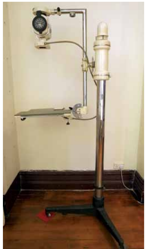
FIG. The Mobile Philips Metalix diagnostic X-ray machine, donated by Dr Hans Tang to the Hong Kong Museum of Medical Sciences in 1996, showing the X-ray tube mounted on one end of the mobile arm and the cassette holder (black plate) on the other end
