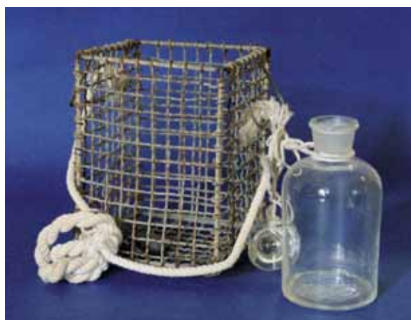
FIG 1. A home-made water sampler for testing water quality used by the old Bacteriological Institute
