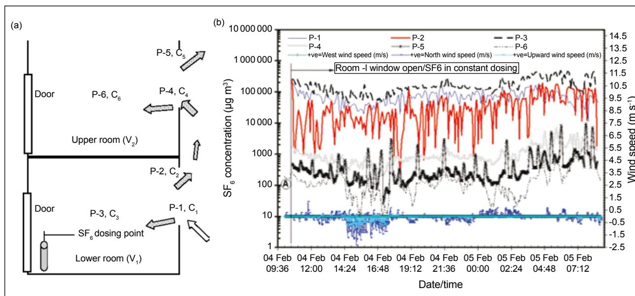
Fig. (a) Tracer-gas dosing and sampling points in the two adjacent floors upstairs and downstairs. (b) Example concentration profiles of tracer gas SF<sub>6</sub> at the six points on two low-wind days
