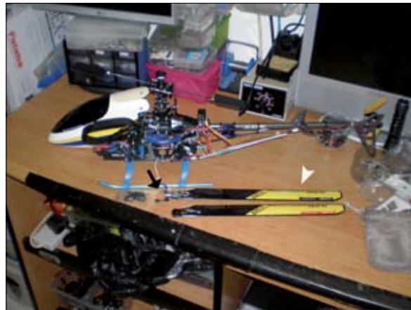
FIG 1. The dislodgment of the blades (white arrowhead) of this radio-controlled helicopter due to breaking of a shaft (black arrow) caused a devastating projectile injury of the eye that resulted in permanent blindness
