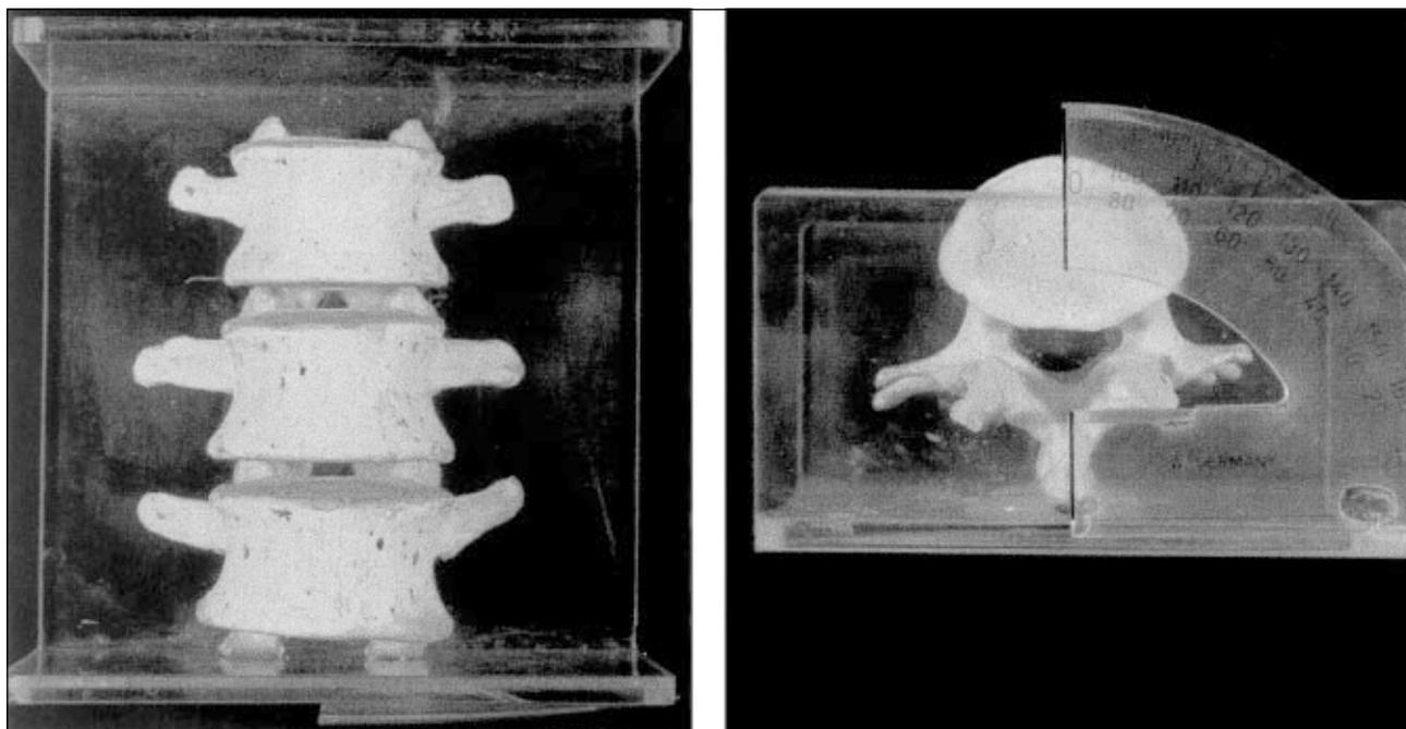
Fig 1. (a) The plastic stand designed for positioning of vertebrae; and (b) rotation of the vertebrae is determined by the line of the spinous process to anterior midpoint of the vertebrae in comparison to the vertical axis
