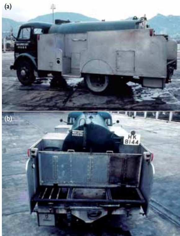
FIG 2. Vehicle designed for night soil collection (a) A large cylindrical tank with two compartments inside and (b) three hoppers at its rear; Reproduced from projection slides donated to the Hong Kong Museum of Medical Sciences Society by Prof SH Lee following his address entitled "The History of Public Health in Hong Kong" to the Society's Medical History Interest Group on 6 February 2010
